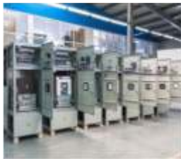
Automatica medium voltage cells for 24kV electrical stations. Transelectrica - Romania.
